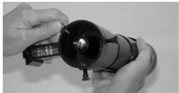
Figure 8b. Pull back on the tensioner and slide the finder scope into its bracket until the O-ring is seated in the bracket ring.
