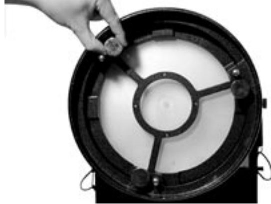
Figure 18. The tilt of the primary mirror is adjusted by turning one or more of the three spring-loaded collimation thumb screws.
