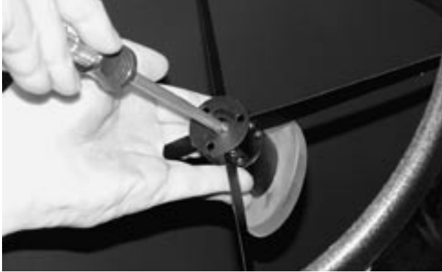
Figure 15. To center the secondary mirror under the focuser, hold the secondary mirror holder in place with your fingers while adjusting the center screw with a Phillips screwdriver. Do not touch the mirror's surface!
