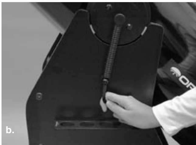
Figure 7. (a) To attach the spring to the base, grip the pull loop with your index finger and pull down on the spring. (b) While pulling down, slip the end ring of the spring over the screw head and onto the narrow part of the nylon spacer, then release the pull loop.
