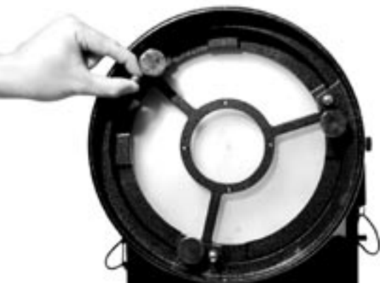
Figure 17. The three thumb screws that lock the primary mirror in place must first be loosened before any adjustments can be made.
