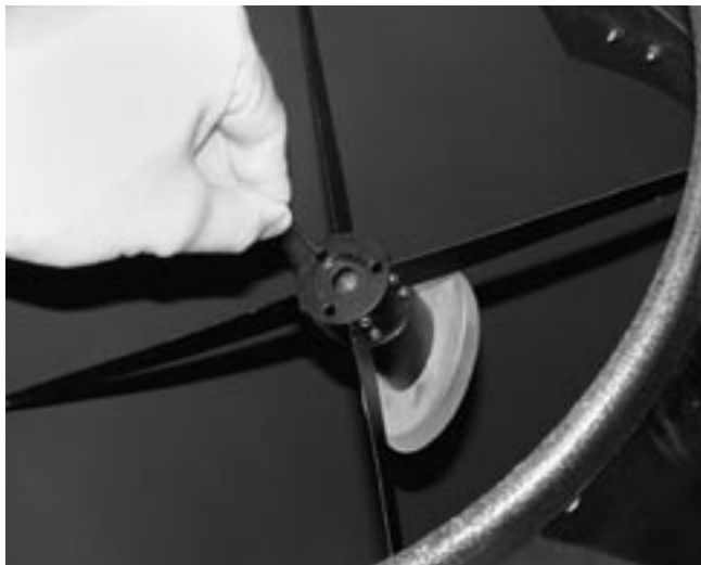
Figure 16. Adjust the tilt of the secondary mirror by loosening or tightening the three alignment screws with a 2mm hex key.
