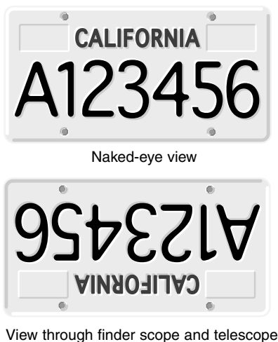
Figure 11. The view through a standard finder scope and a reflector telescope is upside down. This is true for the SkyQuest and its finder scope as well.
