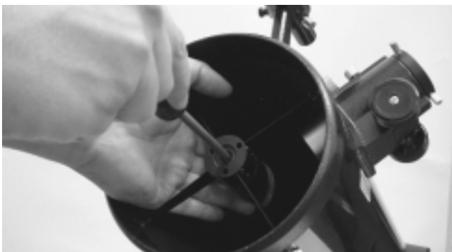
Figure 13. To center the secondary mirror under the focuser, hold the secondary mirror holder in place with one hand while adjusting the center bolt with a Phillips screwdriver. Do not touch the mirror's surface!
