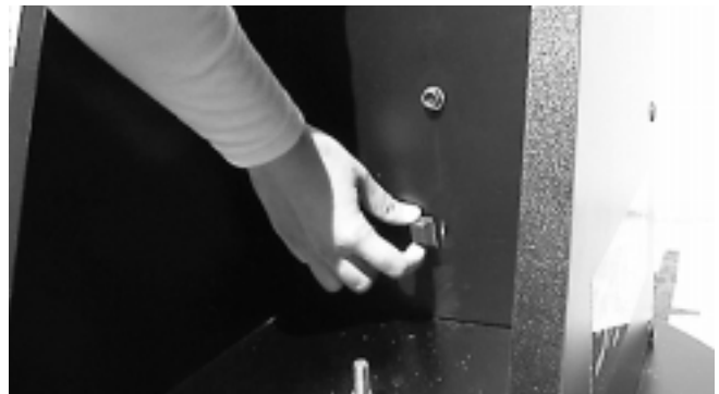
Figure 3. Position the rubber bumper "stop" over the index mark on the inside surface of the front brace.
