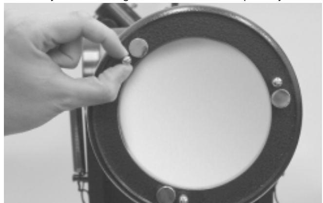
Figure 15. The three small thumbscrews that lock the primary mirror in place must first be loosened before any adjustments can be made.
