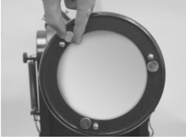
Figure 16. The tilt of the primary mirror is adjusted by turning one or more of the three larger thumbscrews.
