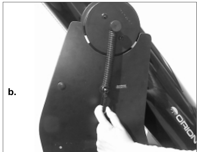
Figure 8. (a) To attach the spring to the base, grip the pull loop with your index finger and pull down on the spring. (b) While pulling down, slip the end ring of the spring over the bolt head and onto the narrow part of the nylon spacer, then release the pull loop.
