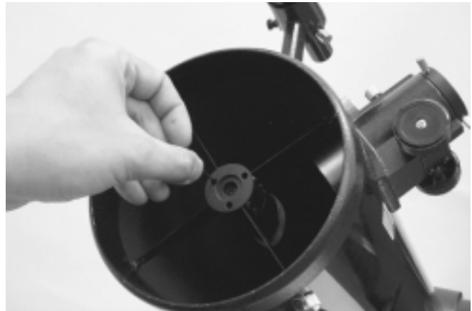
Figure 14. Adjust the tilt of the secondary mirror by loosening or tightening the three alignment set screws with a 2mm hex key.
