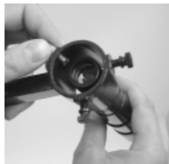
Figure 6b. Inserting the finder scope into the finder scope bracket
