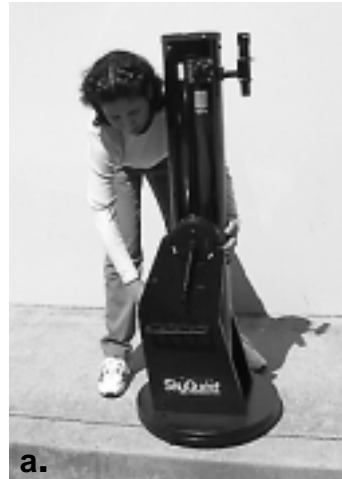
Figure 11. Picking up and carrying the SkyQuest as a single unit (with tube held captive on the base) requires some caution. (a) First, position the tube vertically. Then, grasp the handle on the base with one hand while supporting the tube with the other. (b) With knees bent, slowly lift the base while supporting the tube with one hand. This ensures that the tube will not swing down and impact the ground. (c) As you lift, the whole assembly will tilt down, becoming nearly parallel with the ground, at which time you can let go of the tube with your supporting hand. Make sure you are comfortable with the weight of the whole assembly before attempting to carry it!
