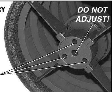
As you adjust each of these screws you will need to make equal counter-adjustments to the other two. In other words, as you tighten one screw you will need to loosen, by an equal amount, the other two. The opposite is also true. If a screw is loosened, the two opposing screws should be tightened. When the process is complete you should have equal tension on all three screws.
