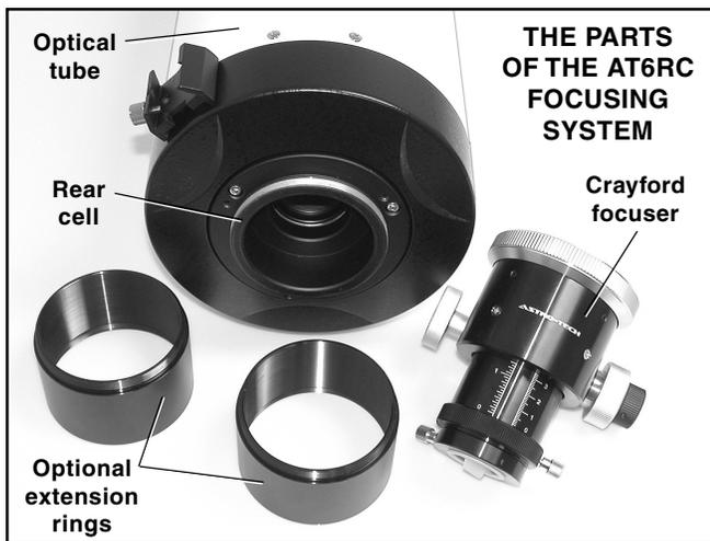
optional Astro-Tech 3.7" diameter extension rings (available in both 1" and 2" lengths) thread in place securely to provide a very strong and rigid mount that holds the focuser at the proper spacing from the scope body to suit your particular camera's requirements.
