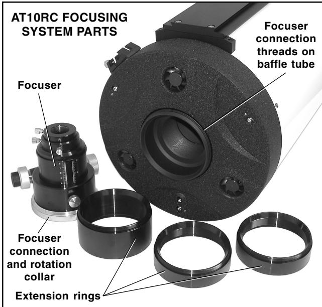
**Components of the Focusing System:** Your AT10RC has an external non-vignetting 3.3" Crayford focuser with a thread-on adapter that steps down from the 3.3" drawtube to a 2" compression ring accessory holder. There is also a separate 1.25" compression ring accessory adapter that can be slipped into the 2" accessory holder. These allow you to use either 1.25" or 2" accessories with no other adapters needed.
