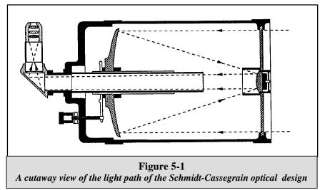
The optics of the CPC have Starbright coatings - enhanced multi-layer coatings on the primary and secondary mirrors for increased reflectivity and a fully coated corrector for the finest anti-reflection characteristics.
